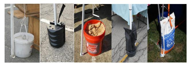
Buckets filled with cement or sand and tied to each corner of the tent with a rope. It is **NOT** sufficient to place the can on the feet of the tent. Canvas bags filled with rocks or sand. **NOTE**: These filled bags usually do not weigh 40 lbs each and must be doubled up (two weights per leg) or combined with other weights.
